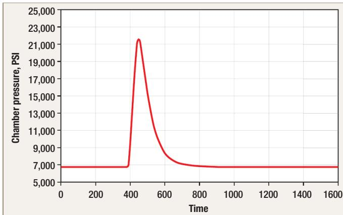
**Fig. 3. Typical pressure-time curve generated for a 22 long rifle**
