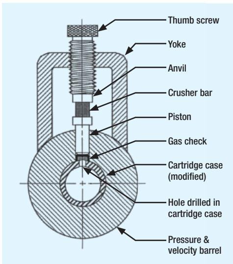
**Fig. 5. Copper-crusher bar test assembly<sup>(1)</sup> (modified by the author)**
