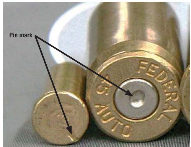
**Fig. 2. Rimfire (left) and center-fire (right) cartridges showing pin marks<sup>61</sup>**
